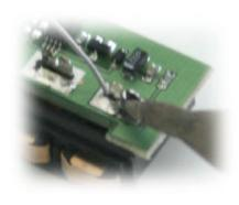
6. Weld the new chip using the wire solder included in our Soldering Kit
