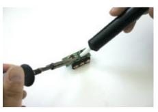
2. Desolder the OEM chip from the connector using our Soldering Kit (code KITSALD)
