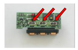
1. Take from the cartridge the OEM chip with the connector
